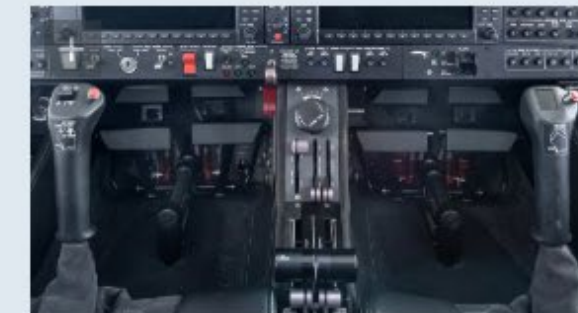
Electrically operated, adjustable rudder pedals for pilot & co-pilot.
