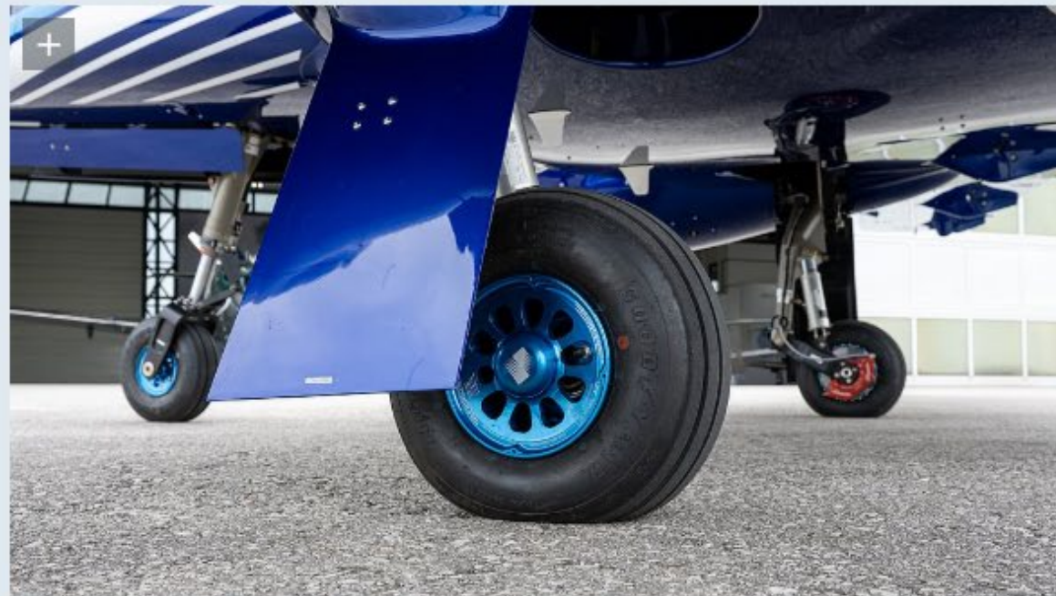
Optional Beringer brakes with SensAIR provide real-time tire pressure and temperature to your smartphone.
